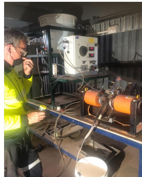
Magnetic separation of chromite
